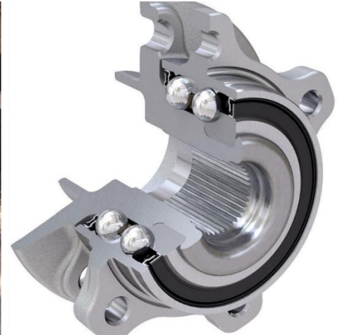
Figure 2: Improved performance of the wheel bearing. From the unlubricated plain bearing to the lifetime-lubricated double-row angular contact ball bearing in back-to-back arrangement with form fit connection to the cardan shaft. (Copyright left: public domain, right: [2])
