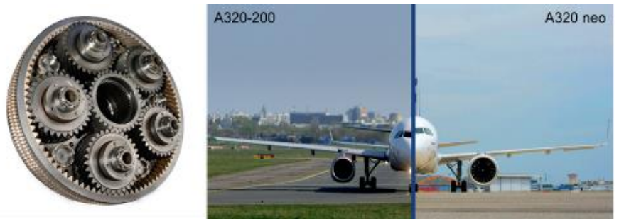
Figure 6: Geared turbofan - planetary gear stage (left) and comparison of Airbus A320-200 and Airbus A320 neo (right). Copyright left: Pratt & Whitney, right: public domain (A320-200), Airbus (A320 neo).
